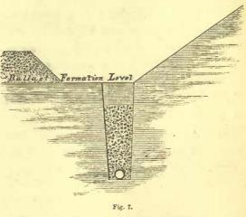
adopted in the formation of underdrains: they are placed, as a rule, immediately at the foot of slopes; formed with drain pipes and the trenches filled with ballast to within a foot of the surface. In rock cuttings, provision was made for carrying off the water by shallow trenches on both sides, as shown in figure 6, so as to keep the track perfectly dry.
